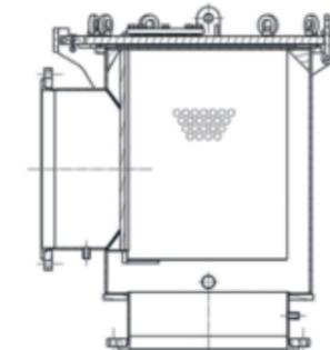
The perforated basket can be made from EUCARO® 10, stainless steel or alternative from steel powder coated, as well as round or square perforation.
