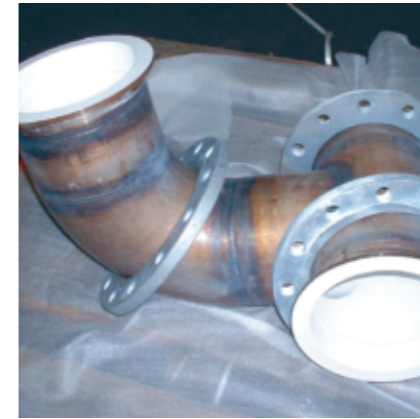
Powder coated pipeline
