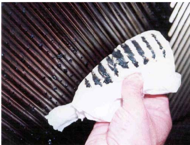
Figure 2: Tar deposits on a plate of a plate and frame heat exchanger using quench water
