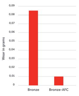
Endurance test 6 hours at a surface pressure of 9 MPa / 1m/s Rotary tribometer (specimen: ring/disk)
