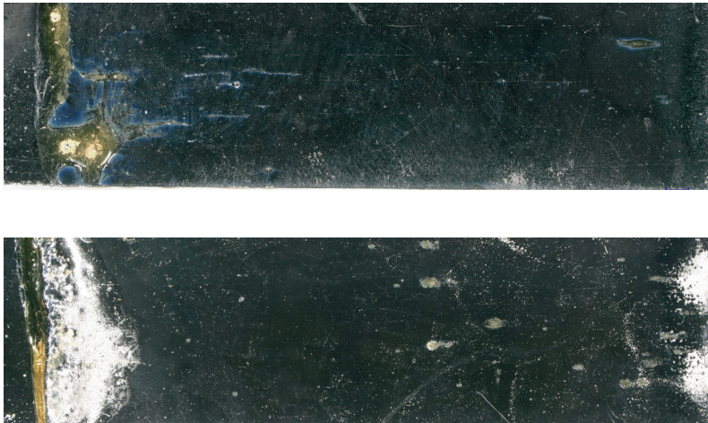
Fig. 8: Wieland-K75 (CuCrSiTi) 0.4mm with 2 - 4 \mu\text{m} thick hot-dip tinning after carrying out the solder bath test according to DIN EN IEC 60068-2-20 with leaded solder SnPb40 (top) and lead-free solder Sn96.5Ag3Cu0.5 (bottom)
