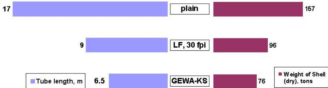
Figure 12. Propane Refrigerant Condenser. Comparison of Plain, LF and GEWA-KS Tube
