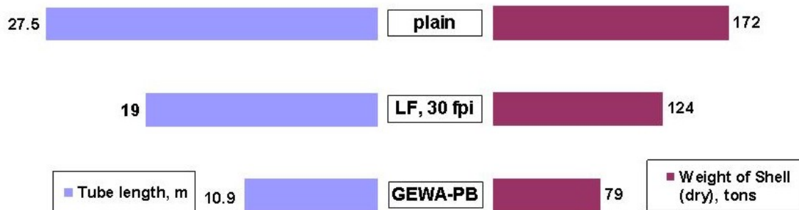
Figure 11. LP/MR Propane Refrigerant Chiller. Comparison of Plain, LF and GEWA-PB Tube
